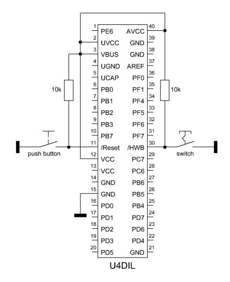
Without firmware, the module always will enter the bootloader. It will respond as "Atmel device" at the personal computer. At the first plugging, it is asked for a driver installation. You have to use the LibUSB-Win32 drivers, which are coming with the "Atmel Flip" installation package.
