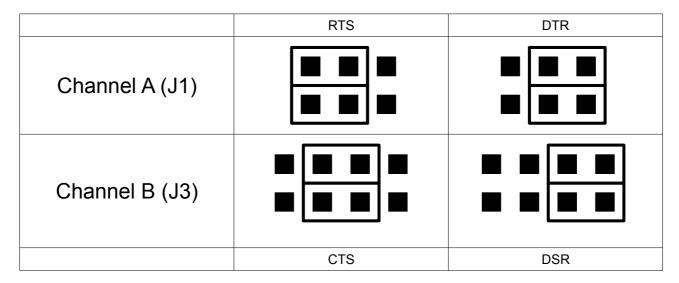
**Hint:** For J2 always a jumper has to be set between pin 1 and 2.
